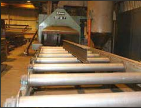
Grit blasting of steel
